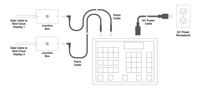
If your shot clock package includes a ScoreLink RF Communications system, the power receptacle may be the only consideration on the control console side of the installation process. For details about ScoreLink, consult the documentation that ships with the product. Otherwise use the stereo patch cables to plug the console into the junction boxes.
